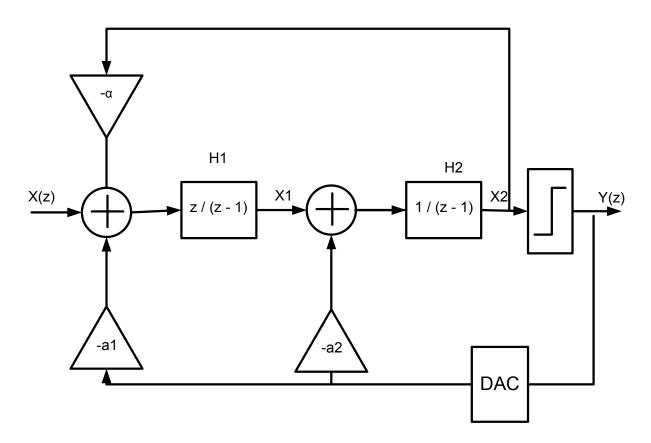
$$Y(z) = z^{-1}X + [1 - (2 - \alpha)z^{-1} + z^{-2}]E/1 - (2 - \alpha - \alpha)z^{-1} + (1 - \alpha - \alpha)z^{-2}$$
